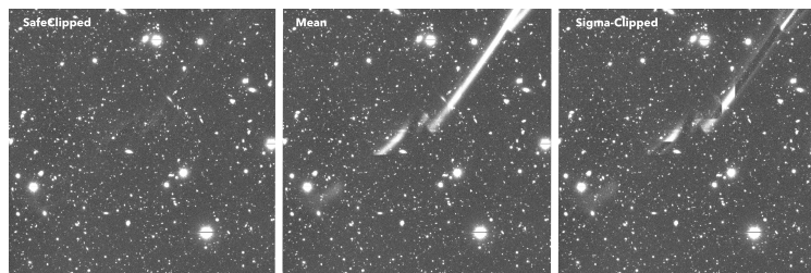
FIGURE 2: A “SafeClipped” (left), mean (middle) and sigma-clipped coadd (right), from ticket HSC-1166. The safeClip algorithm performed well on large, non-overlapping artifacts like these. It solved two problems with the sigma-clipped coadds: the visible wings of artifacts and artifacts falling within the 5\sigma (default) threshold with few numbers or epochs. Because SafeClipped used in an intermediate-stage a sigma-clipped coadd with a 1.5\sigma threshold, it could clip artifacts even with low number of visits.
